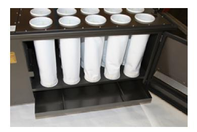
The DDT-XXXX uses a tube filtration system instead of a cartridge filtration system, making it perfect for lighter duty applications. For applications any heavier than wood dust, a cartridge style system (DDC-XXX) is recommended.
